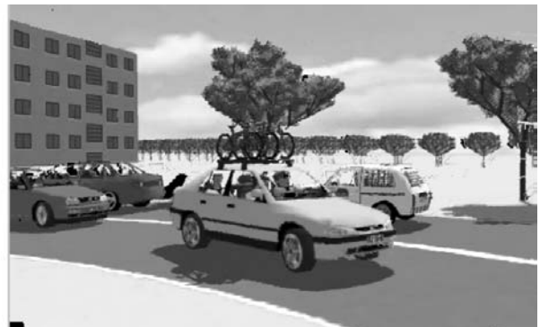
Figure 8/d. Prediction by using all reference views (PSNR = 34.64 dB). The missing pixels are almost covered.
