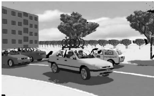
Figure 8/c. Prediction from the nearest left and right reference image (PSNR = 33.45 dB). There are uncovered pixels around the tree on left and the white car.
