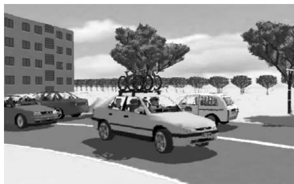
Figure 8/e. The result of the interpolation filtering of the missing pixels on Figure 8/d (PSNR = 36.25 dB)
